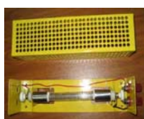
200 watt dump load for 12 / 24 / 36 volt battery banks
